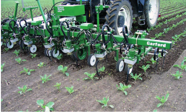
Figure 2.12: Robocrop in action. A camera locates crop plants and controls the weeding device such that crop plants are protected from mechanical in-row weeding. From Garford (2011).
