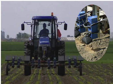
Fig. 2 – The camera unit consisted of camera combined with halogen lamp. During image acquisition were eight such units mounted in front of a tractor.
