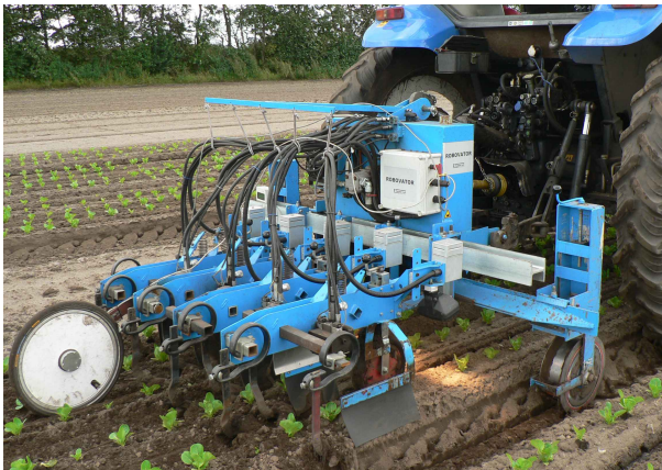
Figure 2.13: The Robovator in action. Halogen lamps were used to provide controlled illumination for the vision system. From visionweeding.com.
