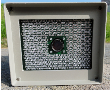
Figure 2.4: Image of the H-sensor. An active illumination system based on LEDs are placed around the bispectral camera. From Piotraschke (2010).
